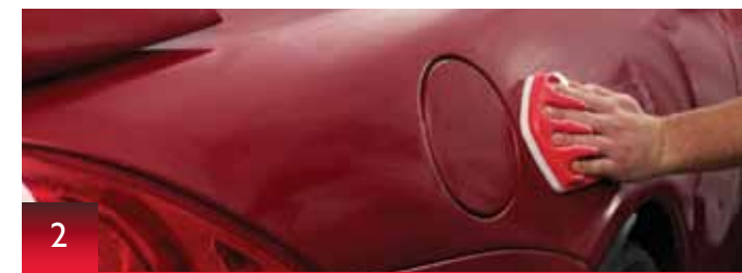
2 Use a light pressure to apply liquid to the car and leave to dry thoroughly for one to two hours to allow resins to cure.
