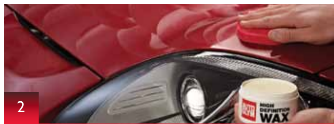
2 When you have applied wax to the whole car, leave to cure for around 15 minutes or more on a cold day.
