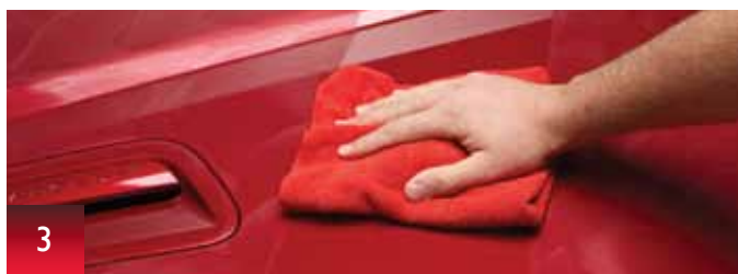
3 Buff to a high gloss with the red finishing cloth supplied, turning it frequently to avoid build-up.
