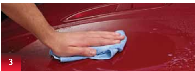
3 Use one of the supplied microfibre cloths to spread the wax, then the other one to buff to a high gloss.
